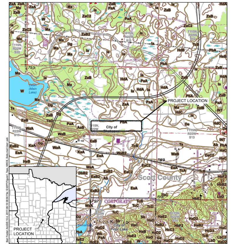
Figure 1 TOPOGRAPHIC MAP WITH SURFACE WATERS AND SOIL TYPES Stormwater Pollution Prevention Plan Scott County, Minnesota
